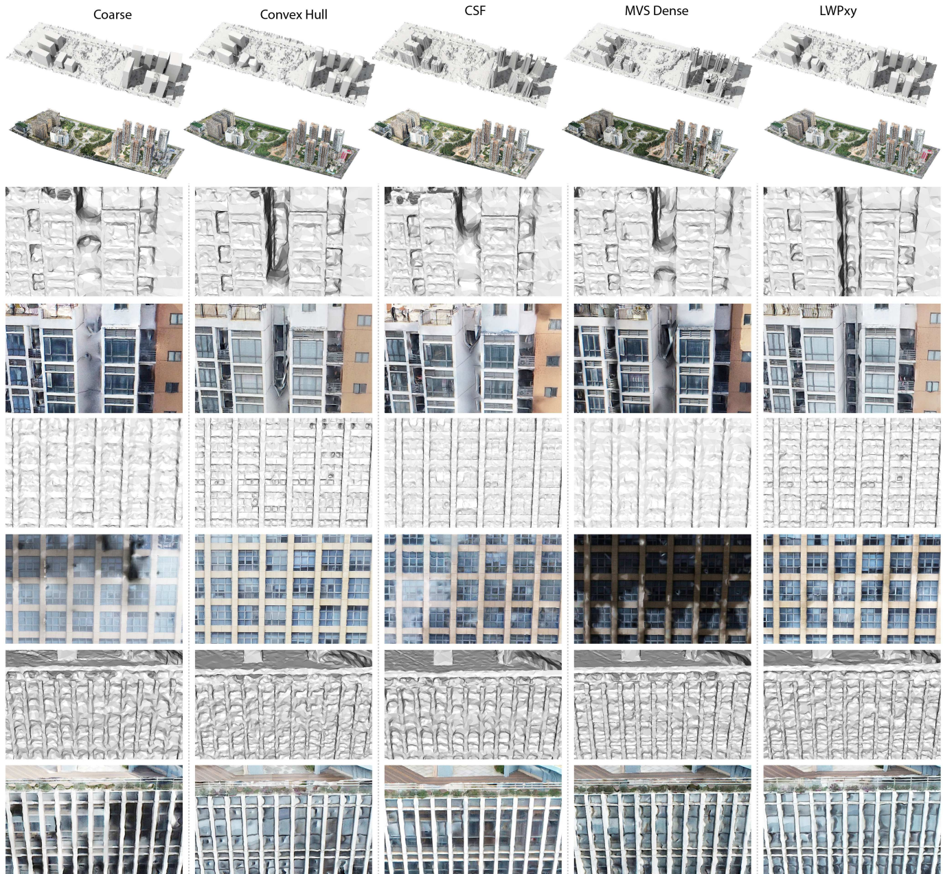
Fig. 10: Visual comparison on the real scene SI-PARK , which demonstrates the effect of different proxy generation methods on the quality of the final reconstruction.
