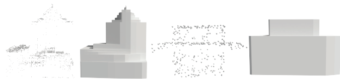
Fig. 11: Our proxy generation method does not deliver the exact geometry of slanted roofs (left) and buildings with a wider top than the bottom (right).
