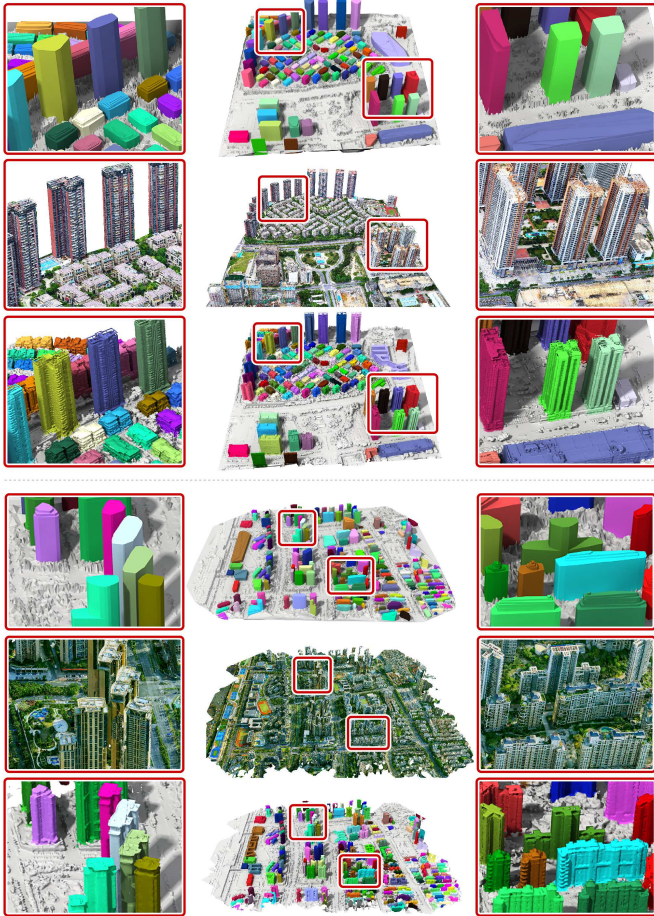
Fig. 7: Instance segmentation results on the Residence-1 (top) and Residence-2 (bottom) real scenes. The three rows of each scene demonstrate the building instance proxies, the final textured mesh of the scene, and the scene mesh with highlighted building instances, respectively. The building instances are randomly colored.
