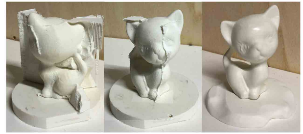
Figure 3: Demonstration of the positional machining strategy. The figure was taken from [NTM*21]. It shows the fabrication of the Kitten model by carving it based on a set of height field patches and subjecting it to manual post-processing.
