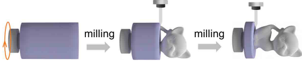
Figure 5: Demonstration of the fabrication process. After assembling the stock on the fixture, we milled it layer by layer along the rotational axis by using the four-axis machine.
