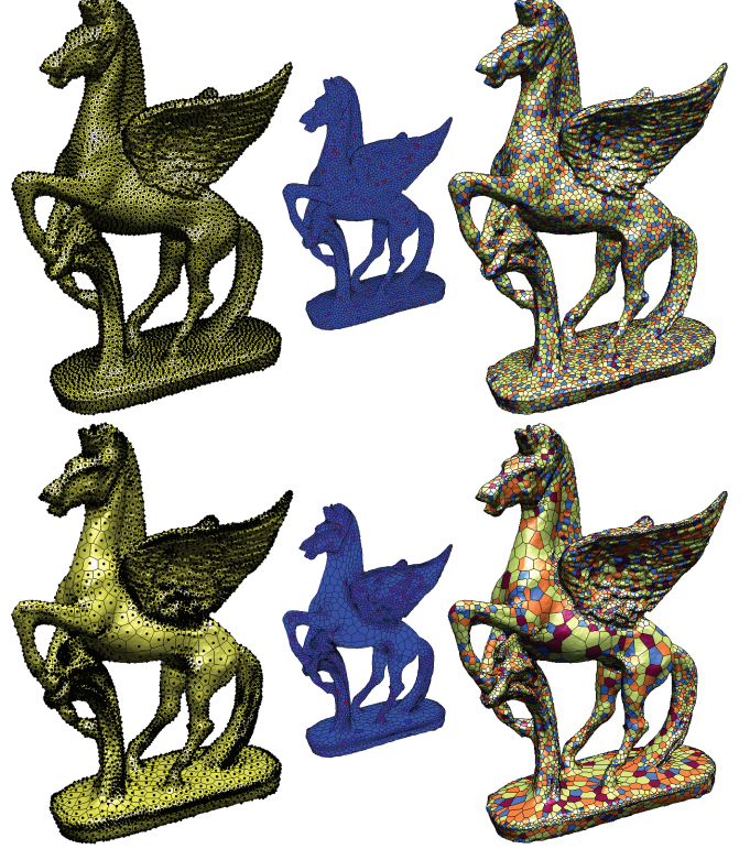
Figure 5: Uniform (top) and adaptive (bottom) sampling on the Pegaso model. The number of sampling points is 10K in both tests. Left: sampled points, middle: quadratic error with respect to the prescribed capacities, and right: restricted power diagram. Different colors indicate different valences of each vertex in the dual restricted regular triangulation. Light green is valence 6 ( v_6 ), orange is v_7 , blue is v_5 , dark blue is v_4 and brown is v_7 .
