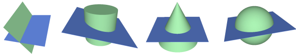
Figure 4: Parametric edges can be calculated as the intersection of primitives (e.g., plane, cylinder, cone, sphere).
