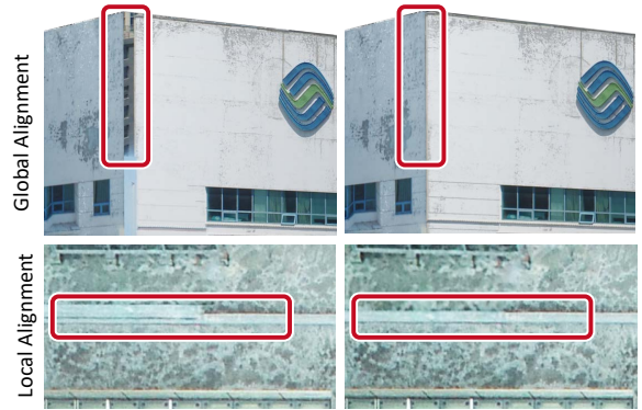
Fig. 5. Left: Texture maps with global and local misalignment before performing line-guided image stitching. Right: After performing image stitching with the adaptive mesh, we can maintain the alignment of line features.
