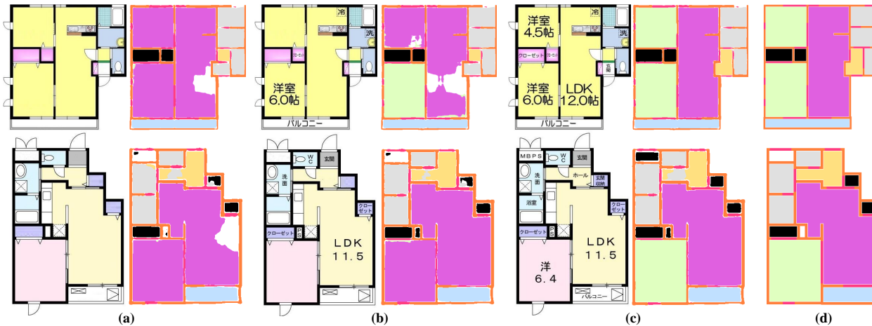
Figure 10. Prediction results of floor plan images without text, fewer text and all texts by our RC-Net. From left to right: (a) Images without texts and predictions of our RC-Net, (b) Images with part of texts and predictions of our RC-Net, (c) Images with all texts and predictions of our RC-Net, and (d) Ground truth.
