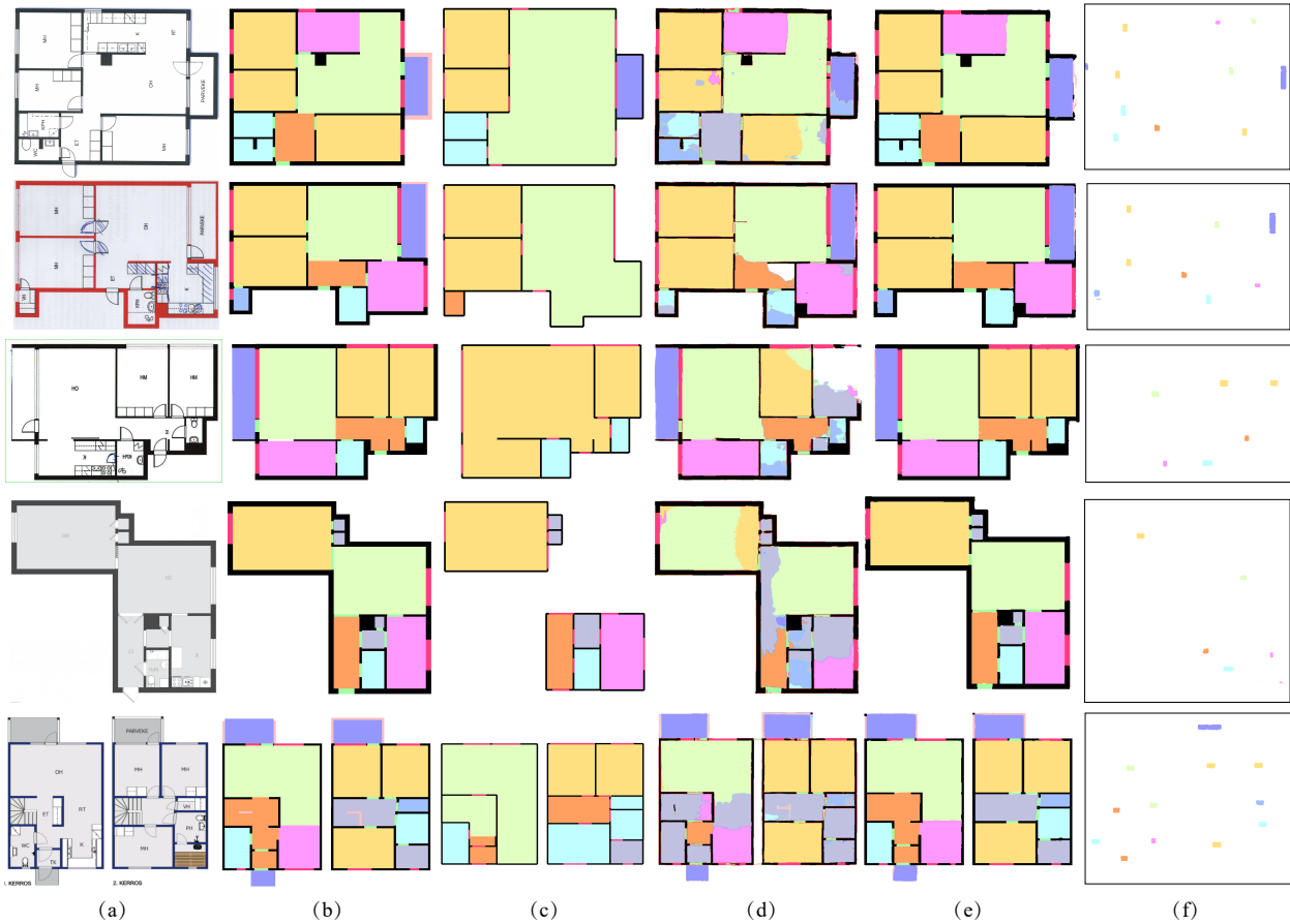
Figure 9. Visual comparison on CubiCasa dataset. From left to right: (a) input floor plan, (b) ground truth, (c) Raster-to-Vector [17], (d) DeepFloorPlan [32], (e) our method, and (f) the text feature mask.
