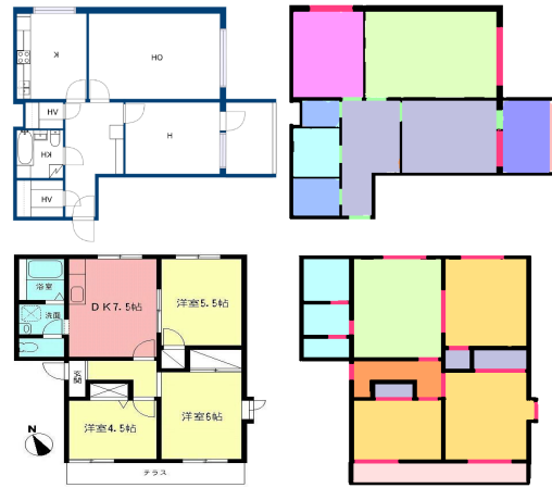
Figure 1. Parsing Floor Plan Images by our RC-Net. Left: the input floor plans that are composed of regular elements and room type texts. Right: our parsing results by elements recognition and room segmentation.
