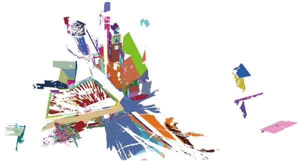
Fig. 3. Primitive shape extraction result for the target point cloud in Fig. 1, where each primitive is randomly color-encoded.
