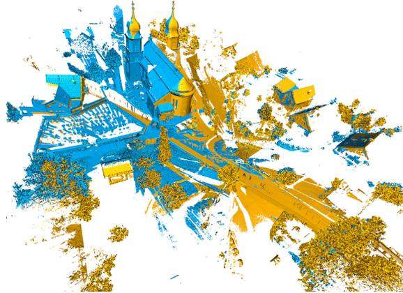
Fig. 1. Point cloud registration of an urban scene from Semantic3D dataset [10] in middle-level structural space, where the target and source point clouds are depicted in blue and yellow, respectively.
