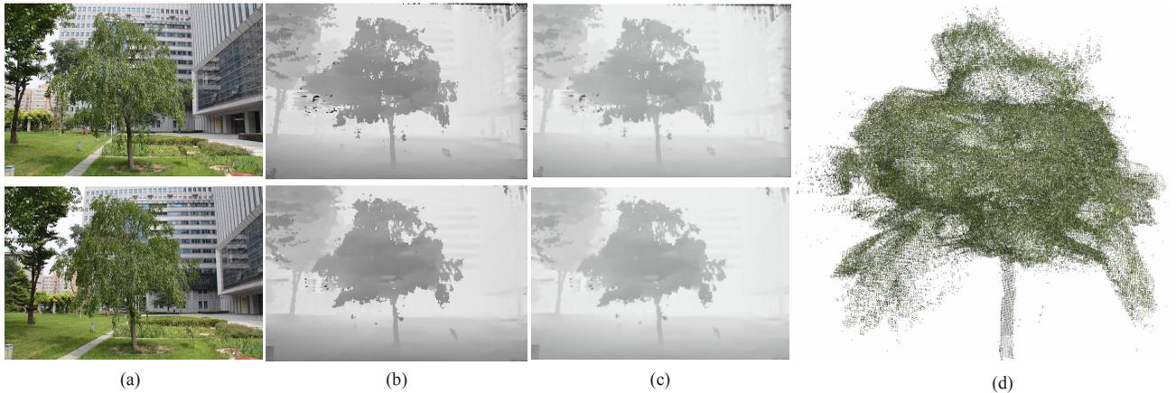
Fig. 3. Key steps of extracting point cloud process. From left to right: input images (a), per-pixel depth estimation by considering the photo-consistency and geometric coherence constraints (b), depth refinement by guided filtering (c), reconstructed point cloud (d). Here we show two views for the depth map computation.
