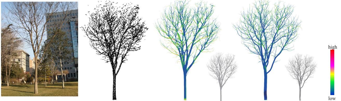
Fig. 14. Quantitative evaluation using a mesh-to-scan distance map. From left to right: 2D photograph, ground truth point cloud, distance map of the approach [9] and distance map of our method.
