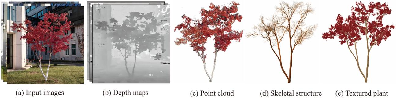
Fig. 2. Overview of our image-based plant modeling system. Given a set of multi-view images (a), we first compute a dense depth map for each image (b), and extract a single point cloud from the depth maps (c). Guided by the point cloud, a rule-based modeling technique is then applied to reconstruct the plant skeleton (d). (e) shows the final plant model with textured leaves.
