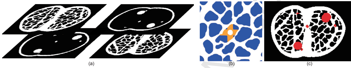
Figure 5: Intersection plane of the transient layer. (a) Normal position and Reverse position. (b) Illustration of the region connection. (c) The intersection of the transient layer.
